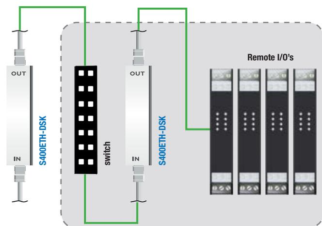
Ethernet Connection with switch placed on Electrical Panel in local
