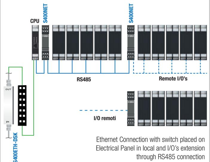
Ethernet Connection with switch placed on Electrical Panel in local and I/O's extension through RS485 connection
